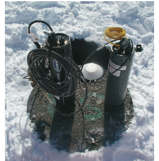
The City of London's Strategic Flow Monitoring Initiative included a move to remote monitoring, using flow meters that transmit data to the municipality's computer system at intervals set by the engineers.
