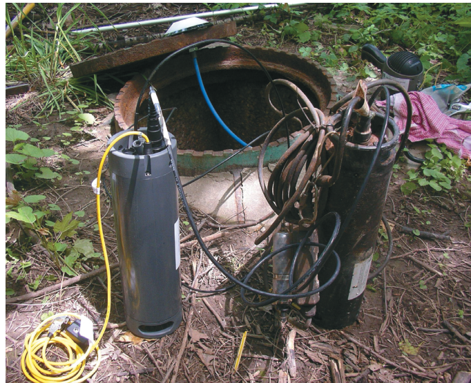
The City of London's Strategic Flow Monitoring Initiative included a move to remote monitoring, using flow meters that transmit data to the municipality's computer system at intervals set by the engineers.
