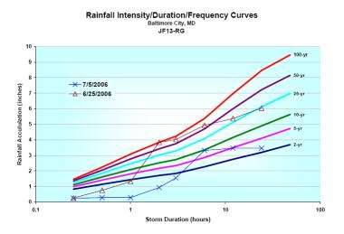
The most significant storm happened on June 25<sup>th</sup> when almost 6 inches of rain fell over a 24 hour period. Although the storm turned out to be a 25 year storm, at one point it had the intensity of a 100-year storm.
