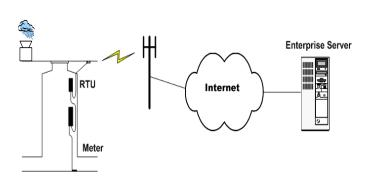
meters and rain and gauges. Referring to the figure above, the RTUs collected and stored the data from the meters and then transmitted the data to the Contractor's Enterprise server.
