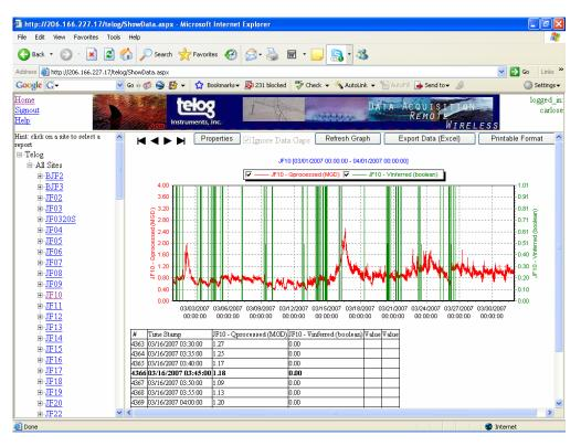
By the last day of each month, each Contractor posted the processed data for the previous month via FTP for Second-Tier QC/QA processing by the City using Telog Tools. Once validated, the data was deemed "Final Data" at the completion of this check. The Second-Tier QC/QA process consisted of the following steps:
