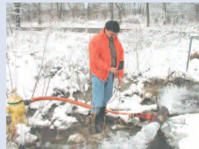
Use your Telog DTU to observe the static pressure at the upstream and downstream hydrants
